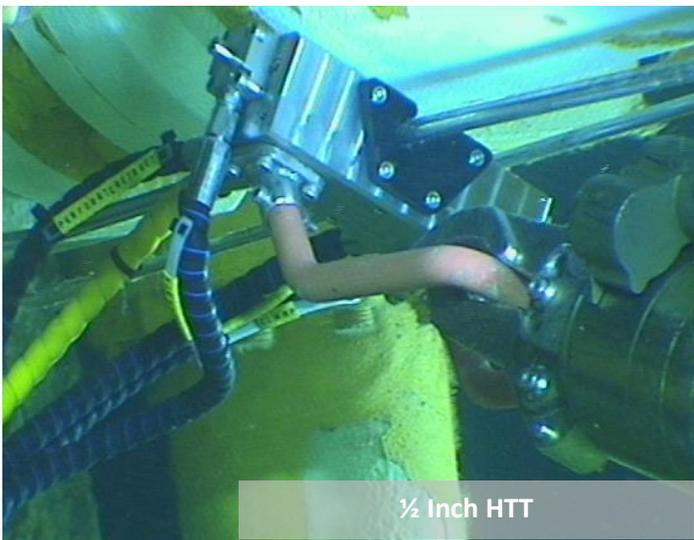
TMT developed and built the first 1/2" version (above) of the highly specialised Hot Tap Tool (HTT) in a very short time. The tools provide fluid injection to the internals of the tree. Importantly, this is done without creating swarf or a coupon that could contaminate the line and potentially cause blockages.
